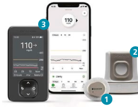
Glucose sensor (1) with applicator (2) and display devices (3) (Dexcom G7)
