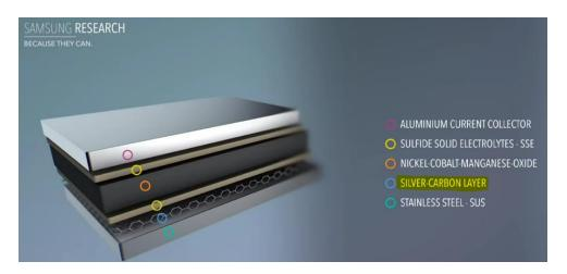
Although not revealed in detail by the company, industry insiders estimate that a single cell will use up to 5 grams of Silver (Ag).
